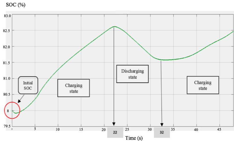
Figure 6. SOC at charging and discharging state
