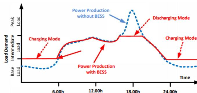
Figure 1. Charging and discharging of BESS in peak shaving application [7]
