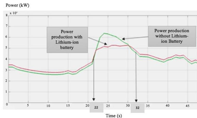
Figure 7. Load demand before and after installing the Lithium-ion
