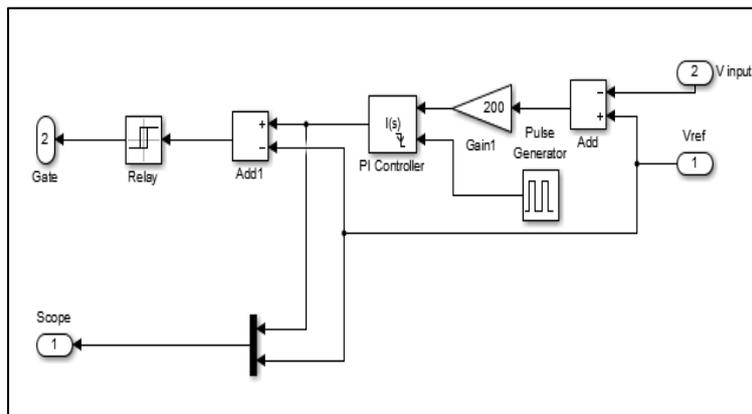
Figure 4. Control system for buck converter
