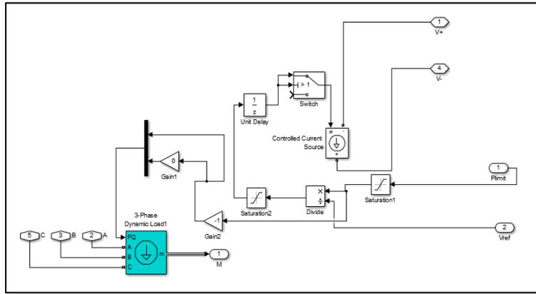
Figure 3. Control system for DC-AC inverter
