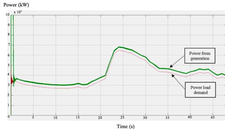
Figure 5. Power production and load demand profile
