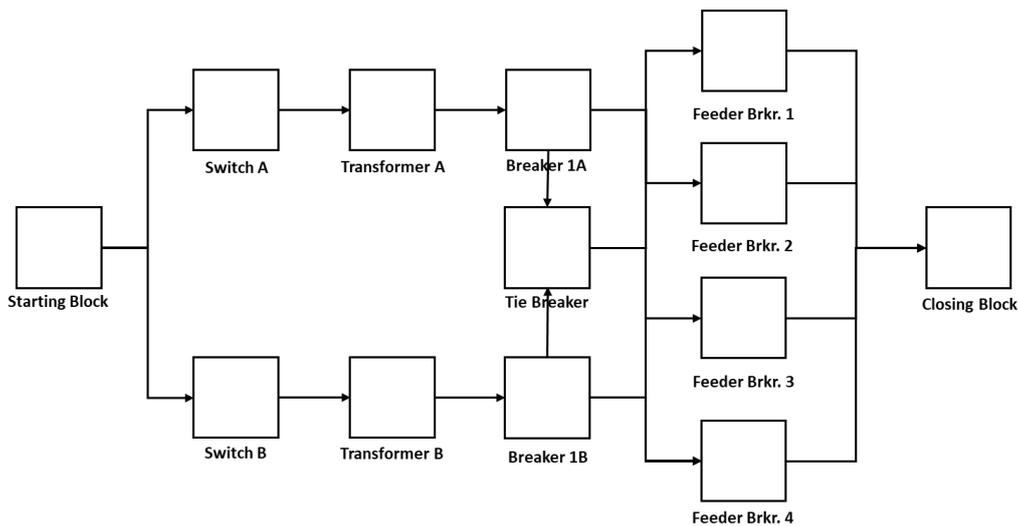
Figure. 7: RBD of a complex substation shown in Figure 2
