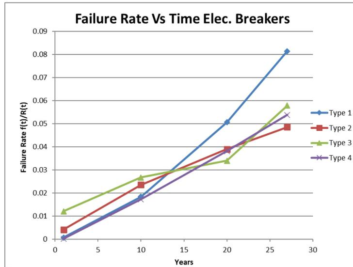
Figure 5. Failure rate curves for different types of breakers
