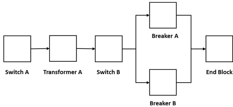
Figure 6. RBD of a simple substation shown in Figure 1
