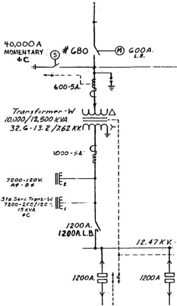
Figure 2. A simple substation configuration
