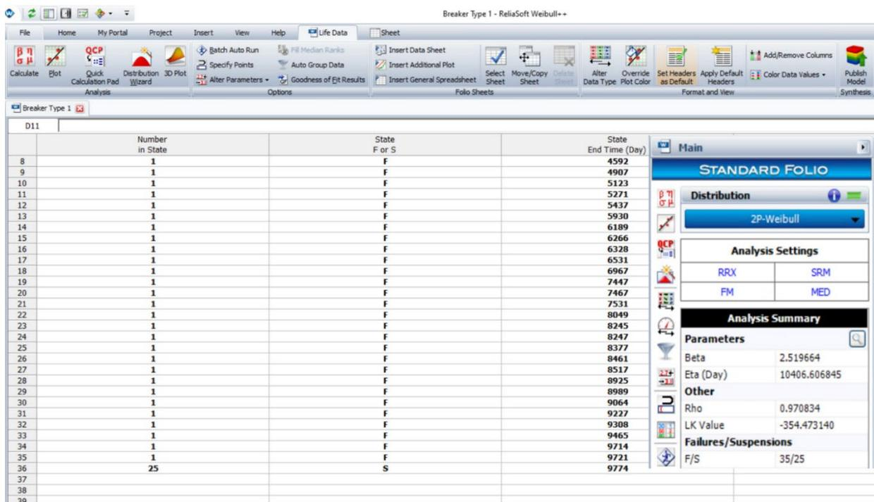
Figure 4. Weibull analysis of Type 1 breaker
