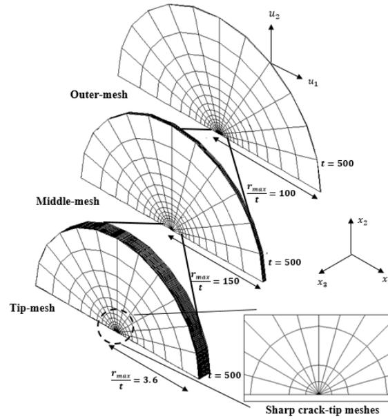
Figure 2. The finite element meshes of boundary layer formulation with a sharp crack-tip
