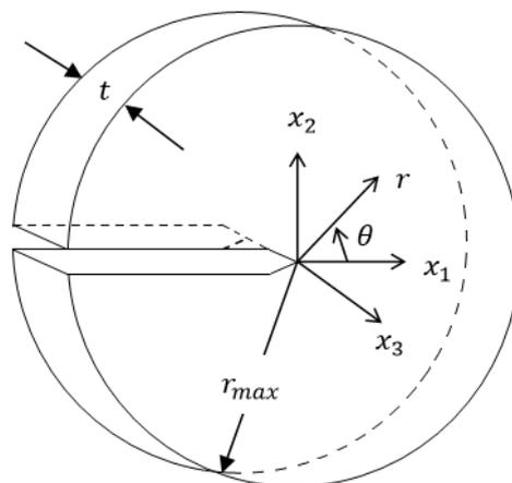
Figure 1. The circular disk representing the near crack front region of a thin plate
