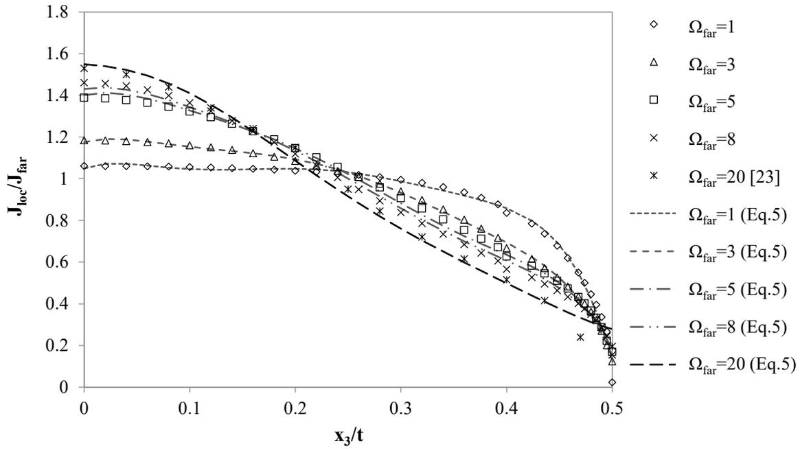
Figure 3. The variation of normalized local  $J$  along the crack front as a function of load levels
