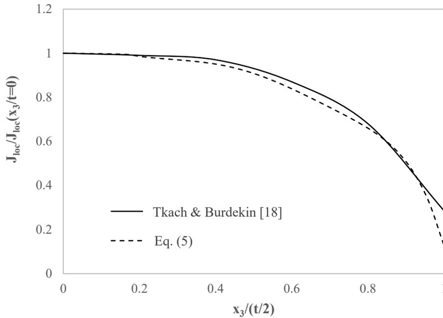
Figure 4. Through-thickness variation of normalized  $J_{loc}$  for  $J_{far} = 100$  N/mm in a 25 mm CT specimen, estimated using Equation (5), and presented by Tkach and Burdekin [18]
