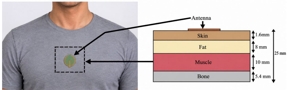
Figure 8. Antenna placement on the multilayer human-tissue heterogeneous model.
