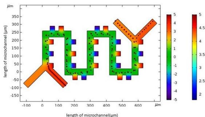
Figure 4(b). The disjunction of blood cells into platelets and red blood cells in a DEP force field when an electric potential of  $\pm 5$  V is applied
