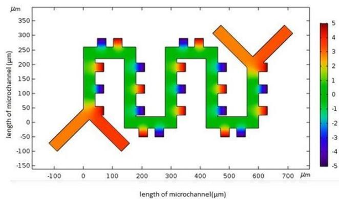
Figure 3(b). The non-uniform electric field distribution inside the microchannel when  $\pm 5$  V is applied
