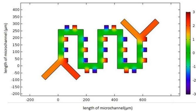
Figure 3(a). The non-uniform electric field distribution inside the microchannel when  $\pm 3$  V is applied
