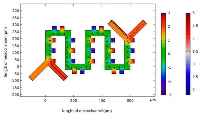
Figure 4(a). The disjunction blood cells into platelets and red blood cells in a DEP force field when an electric potential of  $\pm 3$  V is applied
