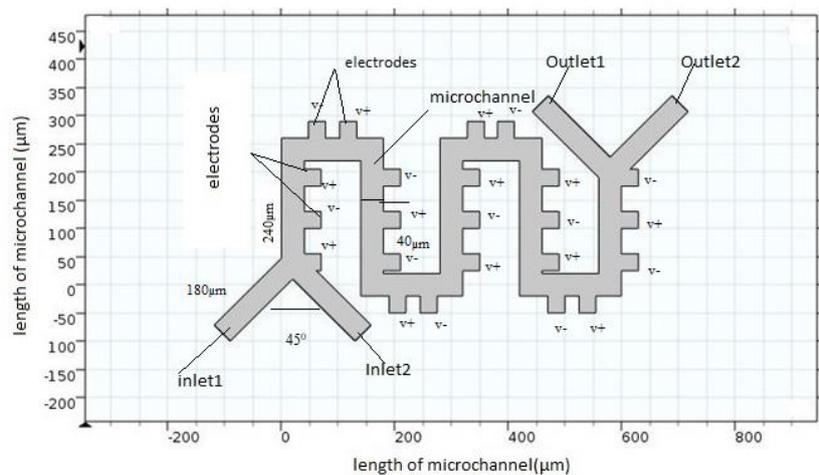
Figure 1(a). Two dimensional geometry of the modeled microchannel
