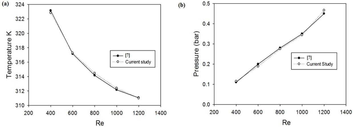
Figure 3. Comparison of (a) temperature with  $Re$  and (b) pressure drop with  $Re$  for plain microchannel
