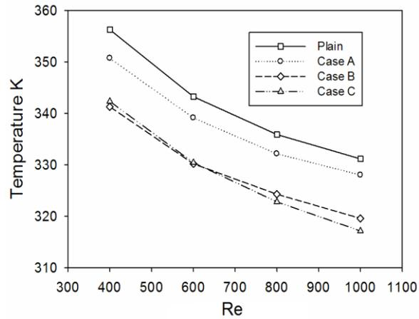
Figure 5. Temperature versus Reynolds number at heat flux  $100\text{W}/\text{cm}^2$
