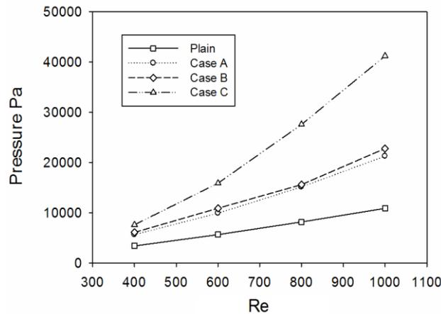
Figure 6. Variation of pressure with Reynolds number at heat flux of  $100\text{W}/\text{m}^2$
