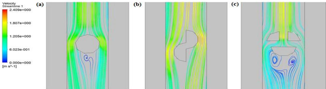
Figure 4. Velocity streamline at  $Re = 600$  (a) Case A (b) Case B (c) Case C
