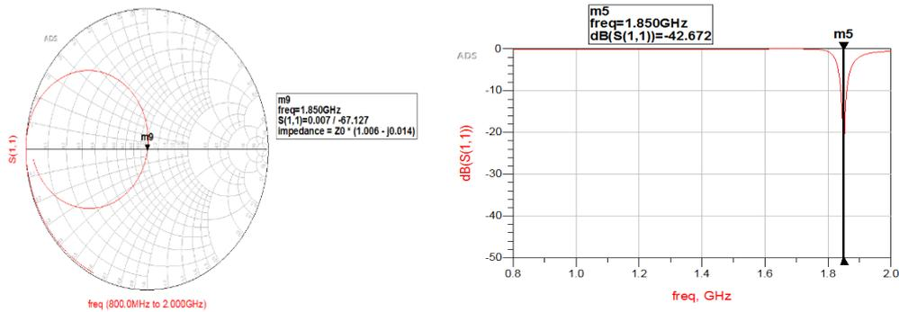
Figure 8. Return loss coefficient ( $S_{11}$ ) response at 1850 MHz frequency after inserted IMN
