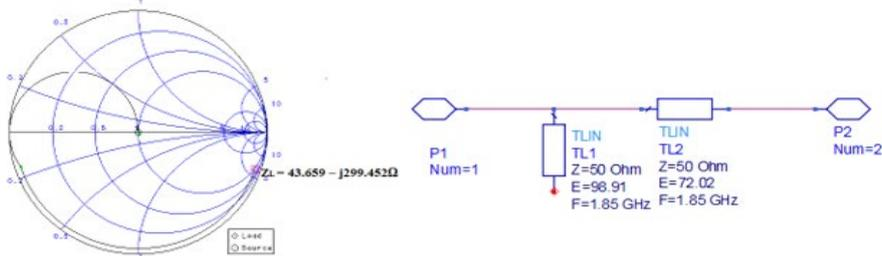
Figure 6. Smith chart for designed open parallel stub IMN at 1850 MHz
