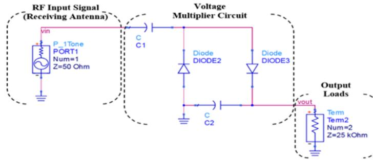
Figure 2. A single stage Villard voltage multiplier circuit
