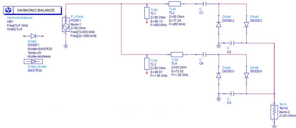
Figure 9. Dual GSM bands RFEH circuit
