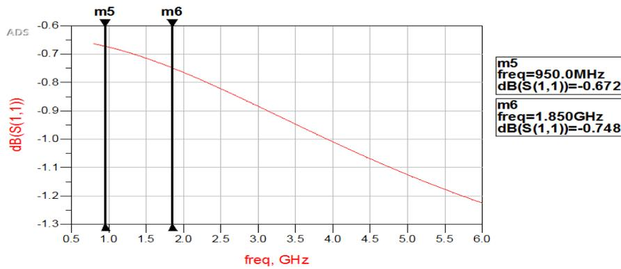
Figure 4. Return loss coefficient ( $S_{11}$ ) response of VMC before matching
