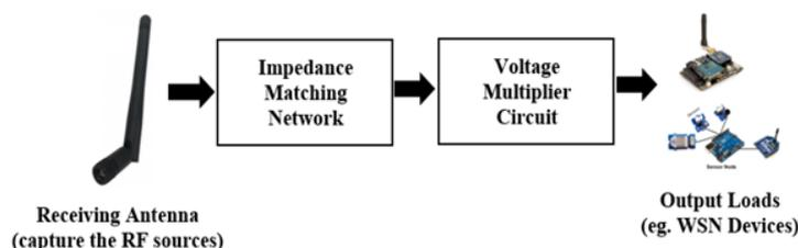
Figure 1. Conceptual block diagram of the RFEH system
