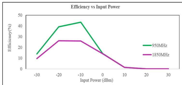
Figure 11. Efficiency of RFEH systems at difference input power signals
