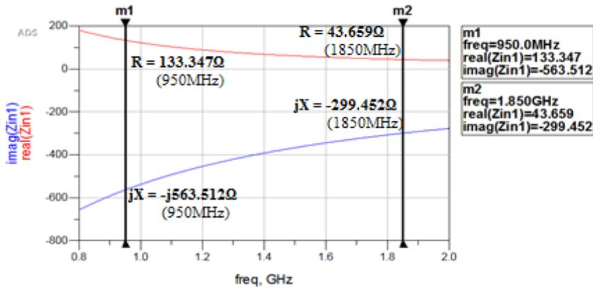
Figure 3. Input impedance of a single-stage voltage multiplier circuit
