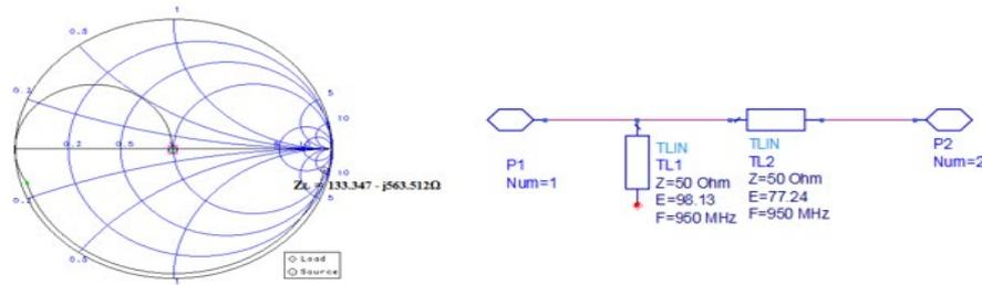
Figure 5. Smith chart for designed open parallel stub IMN at 950 MHz
