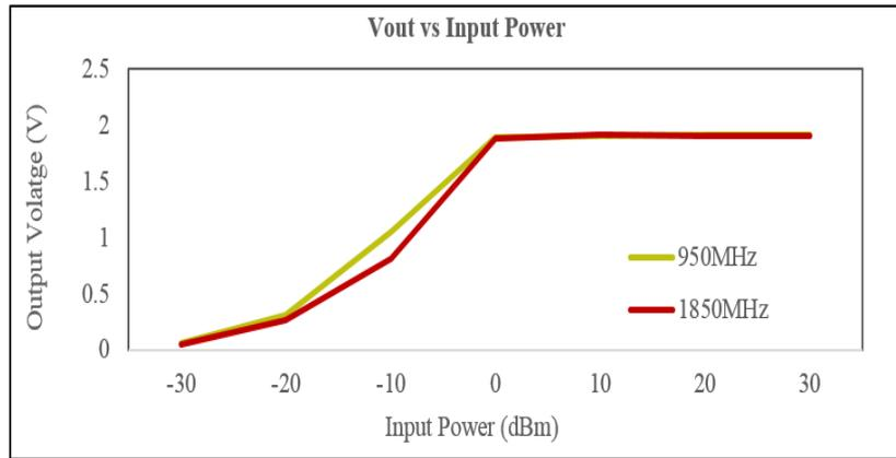
Figure 10. DC output voltage at difference input power signal
