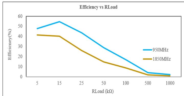
Figure 12. Efficiency of RFEH system at -10 dBm with variant output load
