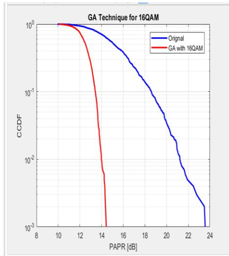
Figure 4. CCDF of 16QAM and 64 subcarrier of OFDM and OFDM-GA
