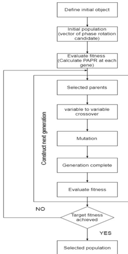
Figure 1. GA flow in OFDM system
