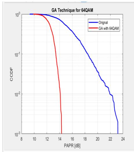
Figure 5. CCDF of 64QAM and 64 subcarrier of OFDM and OFDM-GA
