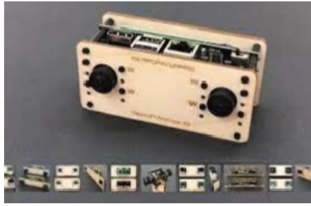
Figure 6. StereoPi stereoscopic camera used in the control system [30].
